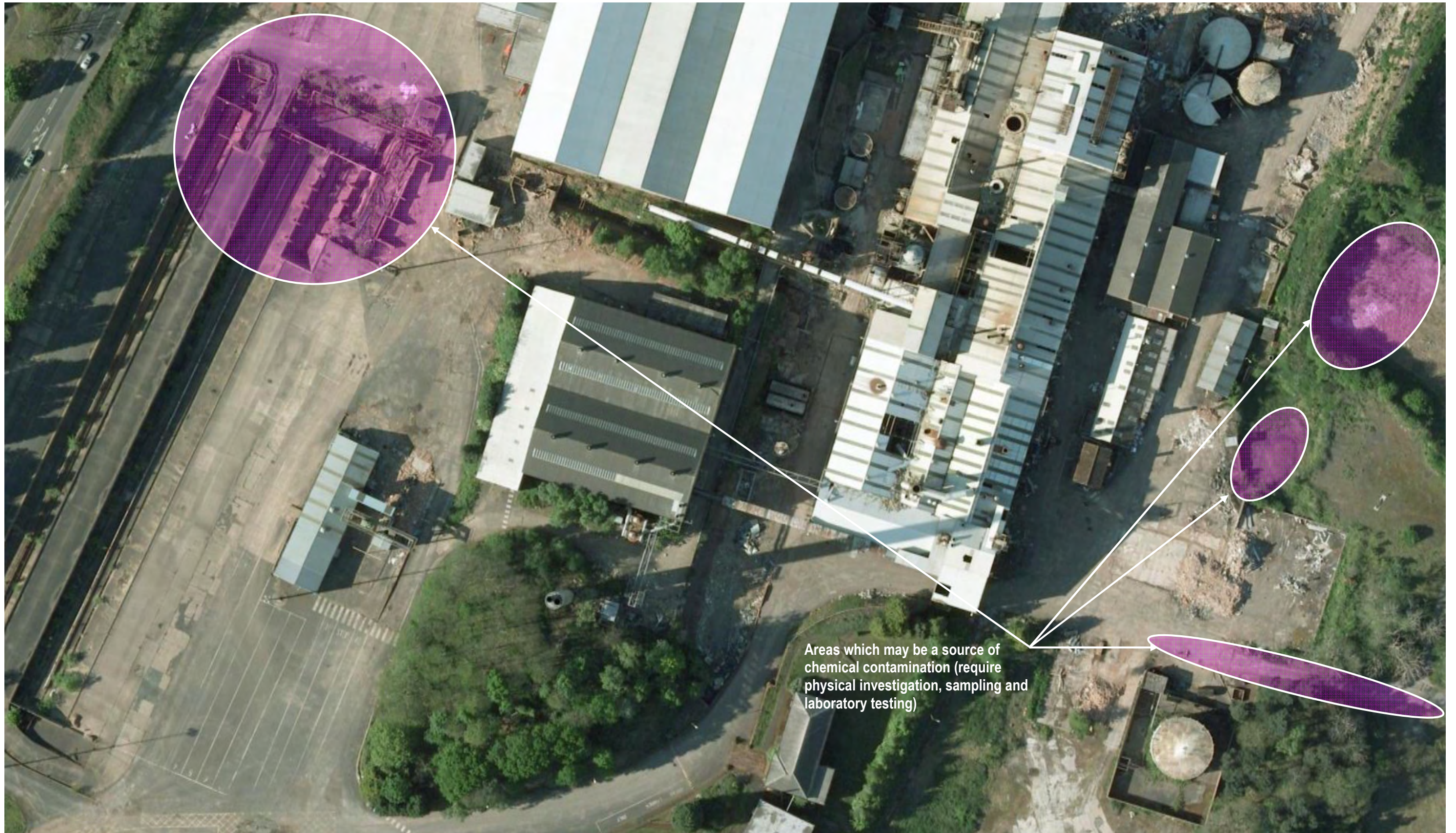
Plate – 6: A portion of the study area; depicting some of the suspicious areas which may source chemical contamination of soil and ground water at the abandoned plant and machinery area of the former 'British Sugar Factory' Site.
